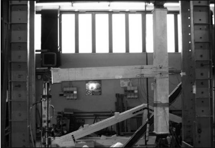
Figure 1 – Typical test on a scaled beam-column joint made of recycled-aggregate concrete, under cyclic loading.
