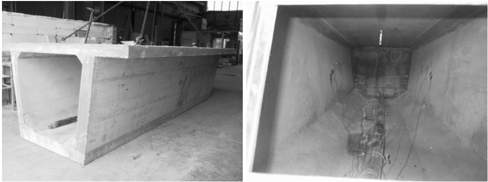
Fig. 8 – Reduced-scale specimen and location of the thermocouples (inside the concrete walls and attached to the tendon); specimen length 500 cm.
