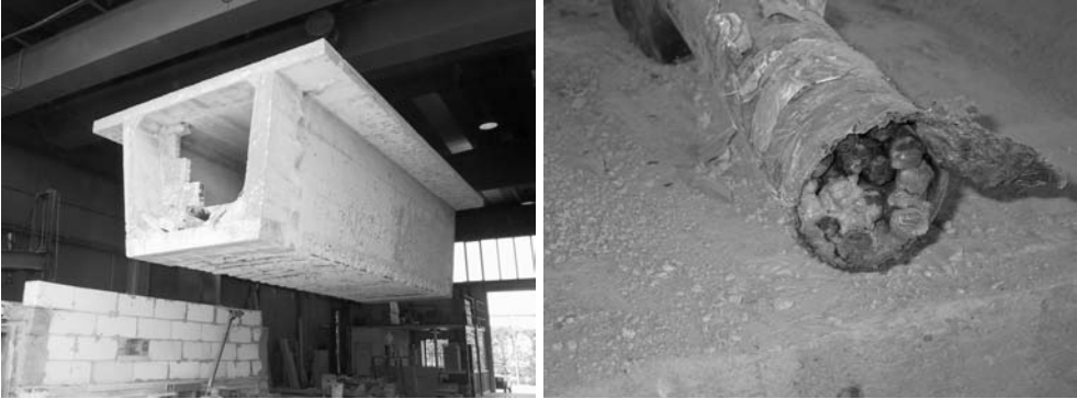
Figure 12 – Reduced-scale specimen after the test in the furnace: (left) concrete spalling along the intrados of the bottom slab; and (right) strands of the tendon in good conditions.
